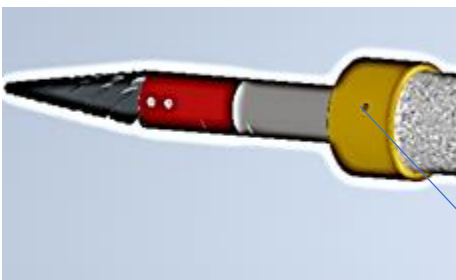
lubrication point / hole
