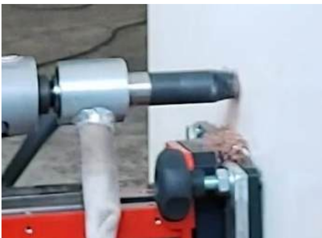
The flat vacuum plate is used like this - on a BD30 fire door
