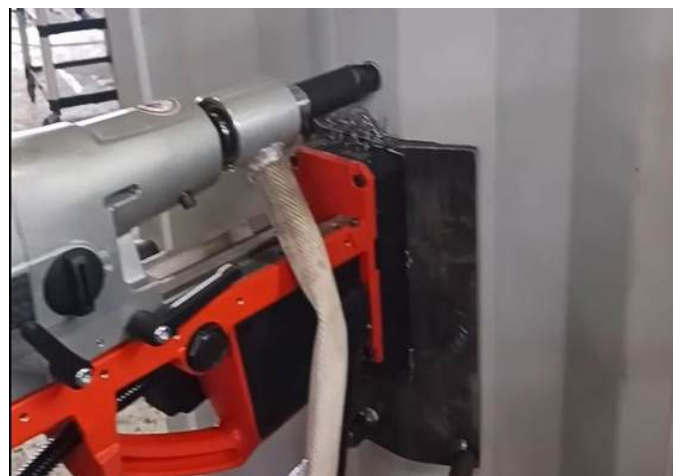
The curved vacuum plate is used like this - on a 20" ISO container
